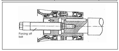
For Fluid Couplings of the 185 and 235 type, the coupligs shaft bore (tolerance F8) allows installation and removal to be carried out manually and this method must be employed.
